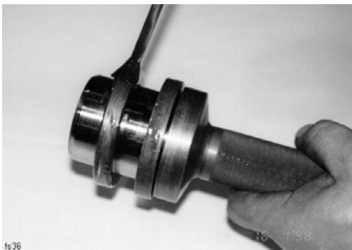
Picture 45 Seal rings being prepared for installation.
