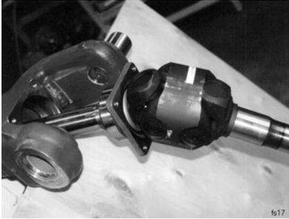
Picture 26 Drive shaft partially out pulled.
