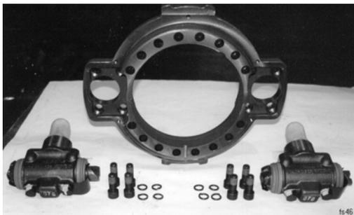
Picture 53 Brake bracket with two expander units with retaining screws
