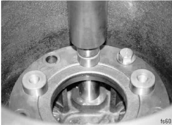
1. Press the planet gear shafts (27) to the hub housing by using a workshop press and a special guiding tool 7 543 049 06 (Picture 16). Use planet carrier cover plate retaining screws to fix the guide tool. Use a special tool 7 543 049 02 (support plate) under the hub housing to prevent the hub housing rolling while pressing the planet gear shafts.
