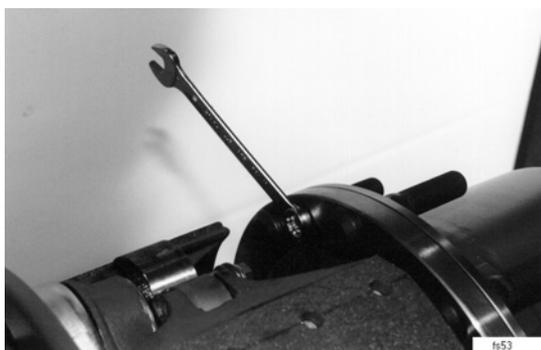
Picture 6 Unscrewing hub housing retaining screws.
